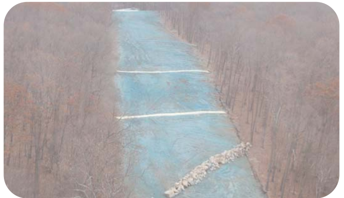
Newtown, CT: An aerial view of the restored right of way after construction of the pipeline loop.
